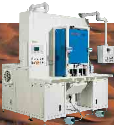
Testing expansion valves
