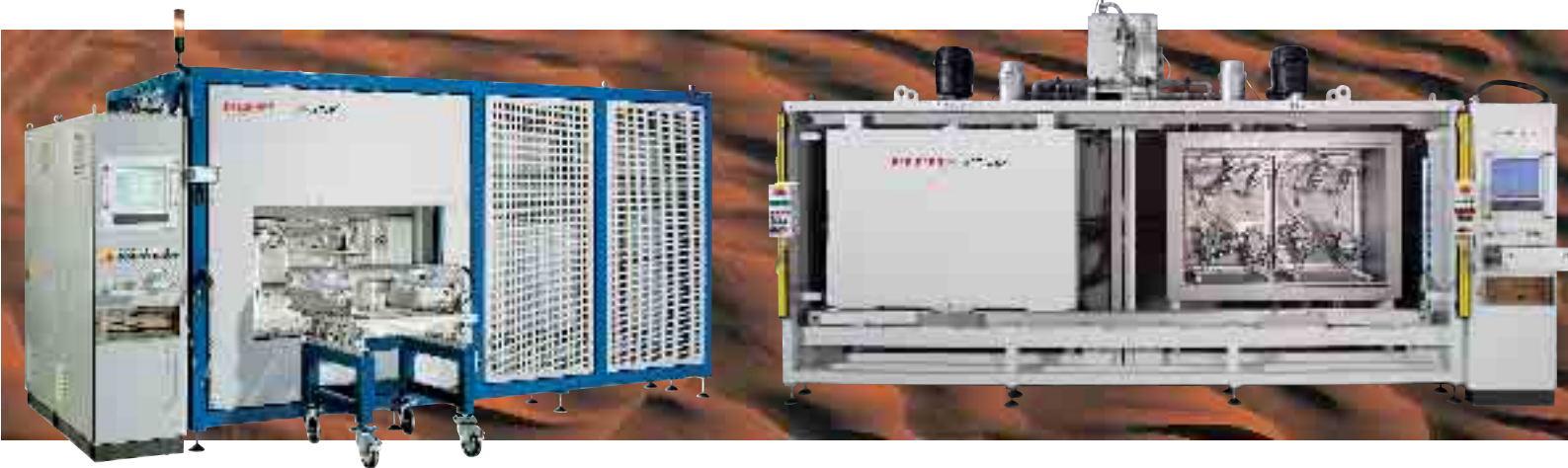
Testing fuel tanks
